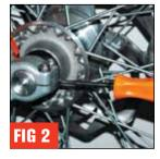
and has a light coating of lube. Slide the axle in, this is where we need to make sure we do not have the forks in a bind. Using a screw driver we need to spread the pinch bolts (FIG 2) this allows the fork leg to move freely on the axel to make sure we have proper alignment. Now tighten pinch bolts per your owner's manual.
